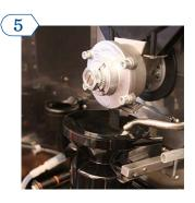
Reinstall the brew funnel, tip the top edge of the funnel under the coffee chute and place the metal pins on the flat springs.
