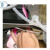
Feed the end of the filter paper through the slit on the under- side of the internal drip tray.
