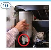
With the dispense elbow in the closed position, reload the hopper with product and reinstall it into the machine. Open the dispense elbow by pushing the tab up.
