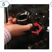
Remove whipping chambers by rotating them counter clock-wise. Remove tops from whipping chambers.
