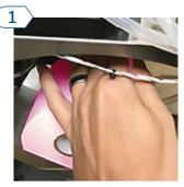
Place a new roll of filter paper in the machine's filter paper compartment located at the bottom left of the machine. Make sure that the end of the filter paper comes from underneath the paper roll. NOTE: If this is done incorrectly, the paper will not advance properly and tear.
