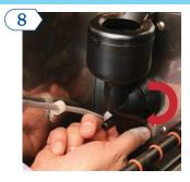
Reassemble whipper chambers parts, reinstall, and rotate tab on whipper base clock wise to the vertical position to lock mixing chamber. <u>Reinstall dispense hoses</u> and elbows to hoppers.
