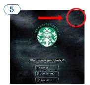
Weekly Cleaning Instructions Once the system cleaning process is complete, advance the filter paper by pressing and holding the upper right corner of the screen (about 15 seconds) until the "Service Access" screen appears.
