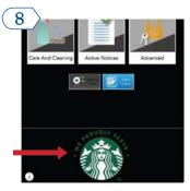
Exit out of the "Service Access" screen by pressing or swiping the Starbucks logo in the center of the screen.
