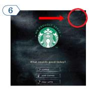
Close the machine door. From the Menu Build screen, press and hold the upper right corner of the screen (about 15 seconds) until the "Service Access" screen appears.
