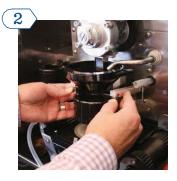
Using both hands, press down on the flat springs located under the metal funnel arms.
