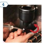
Rotate tab at the base of the whipping chamber counter clock-wise to release the base.
