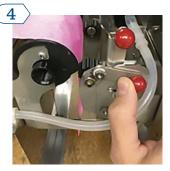
Pull back the red knob of the tractor drive and feed the filter paper between the rubber tractor drive gears, so that the end of the paper is aligned with the machine's internal waste bin or waste chute.
