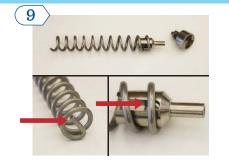
**NOTE:** The slot in the auger drive shaft fits only on one end of the auger wire. See images for correct placement. Failure to reinstall the auger wire correctly will result in product not dispensing.
