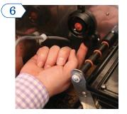
When reassembling parts, be sure to reinstall O-ring on mixing chamber base then rotate tab on whipper base clock wise to the vertical position.
