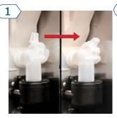
Close the soluble hoppers by turning down the tab on the dispense elbow.
