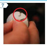
When reassembling the frother disk, align arrow on frother disk with flat on whipper motor shaft.
