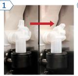
Close the soluble hoppers by turning down the tab on the dispense elbow.
