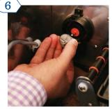
Remove frother disk from shaft by pulling straight out. Rotate tab on mixing chamber base counter clock-wise, and
