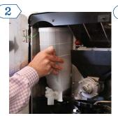
Remove the hopper from the machine.
