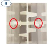
Remove the agitator disk and mixing blades inside the hopper by slightly spreading the hopper walls and pulling the agitator disk shaft ends one at a time from the hopper wall pivots.
