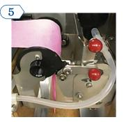
Release the red knob of the tractor drive making sure that the tractor drive's rubber gears are in contact with the filter paper. NOTE: If the tractor drive's rubber gears are not properly engaged with the filter paper, the filter paper will not advance and an "Active Notice" will appear on screen.
