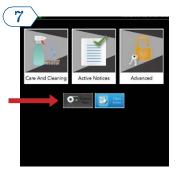
Press and hold the "Advance Paper" button until you hear the tractor drive motor stop. <u>NOTE:</u> <u>Failure to advance the paper after installing a</u> <u>new roll will result in an "Active Notice" stating</u> <u>that the machine is out of paper.</u>
