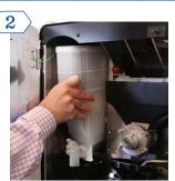
Remove the hopper from the machine. Remove the lid and empty the hopper of product.
