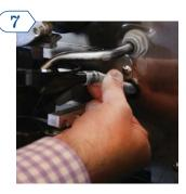
Reconnect the rubber hose by sliding it over the funnel inlet fitting. <u>Ensure that the</u> <u>hose is fully engaged.</u> Close the machine door to resume normal operation.
