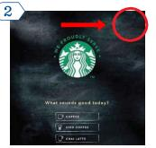
From the Menu Build screen, press and hold the upper (about 15 seconds) until the "Service Access" screen appears.
