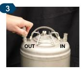
With the collar pulled back, place the connector on the keg's valve labeled "OUT"
