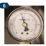
Recheck the pressure reading on the regulator gauge. If necessary, repeat steps 2-6 until proper pressure reading has been reached.
