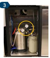
Position the nitrogen tank inside of the kegerator so that the gauges of the regulator are visible. \*
