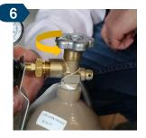
Open the shut-off valve on the nitrogen tank by turning the valve handle all the way counterclockwise.
