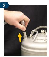
With the connector collar up, pull up on the connector until it disengages from the keg
