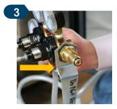
IMPORTANT: Before attaching the regulator to the gas tank, ensure that the gas tank wrench is attached to the regulator connector.
