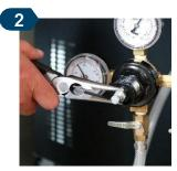
Using pliers, loosen the adjustment nut on the regulator.
