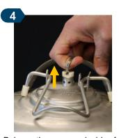
Release the pressure inside of the keg by pulling on the pressure release ring located on the keg. You will hear the pressure being released.
