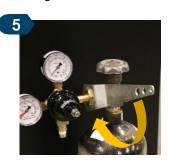
Use the attached gas tank wrench or a standard wrench to completely tighten the regulator's connector to the nitrogen tank.
