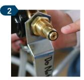
Inspect the nitrogen tank connector to ensure that the O-ring is in place\*
