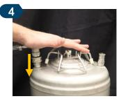
Push down on the top of the connector until the collar drops into place and a "CLICK" is heard \*
