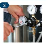
With a screwdriver, turn the regulator adjustment screw clockwise to increase or counterclockwise to decrease pressure levels as need
