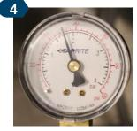
Once the "needle" aligns with 28psi, retighten the regulator adjustment nut
