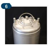
Tilt the keg to ensure that no liquid leaks from the lid. Repeat locking if necessary
