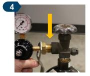
Insert the regulator's threaded nitrogen tank connector into the nitrogen tank fitting, then hand tighten.
