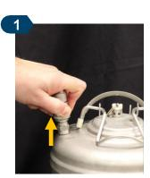
Lift up on the collar around the base of the connector
