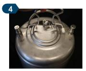
Pull up on the lever until the lid's gasket and the keg opening are aligned
