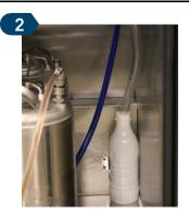
Place the drip tray drainage hose into the drainage container the place the drainage container between the holder bracket in the back of the kegerator
