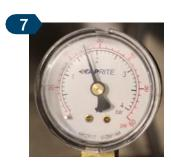
Check the beverage line regulator gauge to ensure that the pressure reads 28psi.
