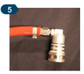
Locate the chrome keg coupler attached to the RED gas hose
