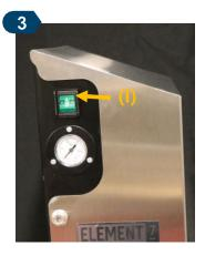
Turn on generator and allow it to run until fully pressurize; approx. 2-5 min.
