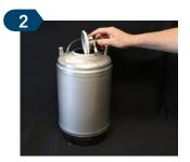
Turn the lid sideways and insert it into the opening at the top of the keg
